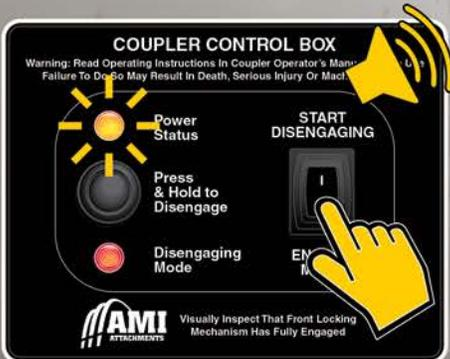
**1.** Start the process by switching the engage mode on. The power status signal indicates that power is on accompanied by a continuous audio alarm.
